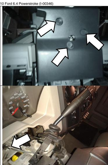
Pop the electrical connector for the *12.* shift lever out of the mounting location on the top of the steering column. Disconnect the shift lever wire from the vehicle.
