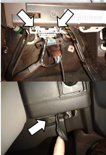
10. Remove the steering column tilt handle rubber grommet and remove handle by removing the T20 screw securing it.
