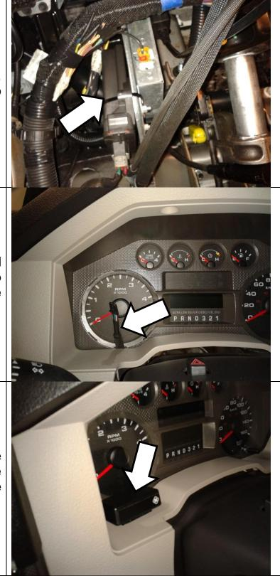
8. NOTE On models without a mileage reset button in the instrument cluster, it is possible to install the display above the shift lever on the right side of the instrument cluster instead of the left. This is left to the customer's preference.
