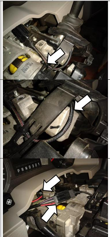
20. Reinstall the lower column cover by installing the three 5.5mm screws. Snap upper half to lower half. Reinstall knee bolster. In-cab portion of the installation should now be complete.
