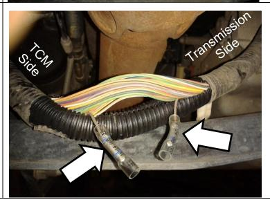
27. Strip the yellow and blue wires from the BD harness and crimp the blue wire into the side that goes to the transmission and the yellow wire into the transmission controller side (frame rail side).
