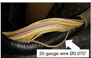
**26.** Cut this wire and strip the ends. Crimp on the supplied heat shrinkable butt connectors.
