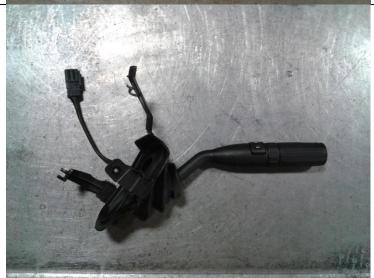
17. Install new shift lever by reinstalling T30 securing screw and the two 5.5mm boot attaching screws. Secure the wire with a wire tie to the plastic wire clip such that the wire will not rub or chafe during use.
