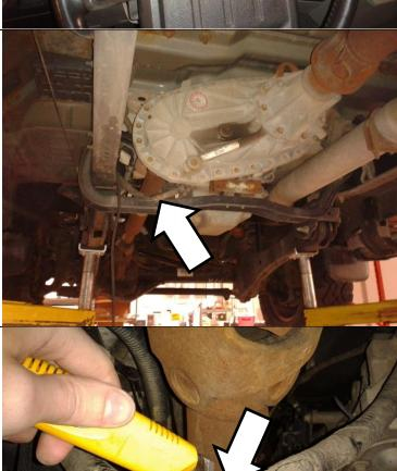
24. Pull wires out of the harness and locate the 20 gauge gray wire with a brown tracer. Use care when locating the wire as there is an 18 gauge wire of the same color for the ISS in this harness.
